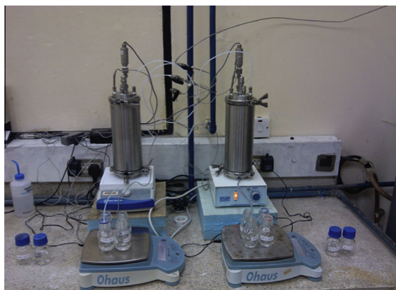
Fig. 4. Stainless steel stirred cell experimental apparatus at the University of Dar es Salaam.
